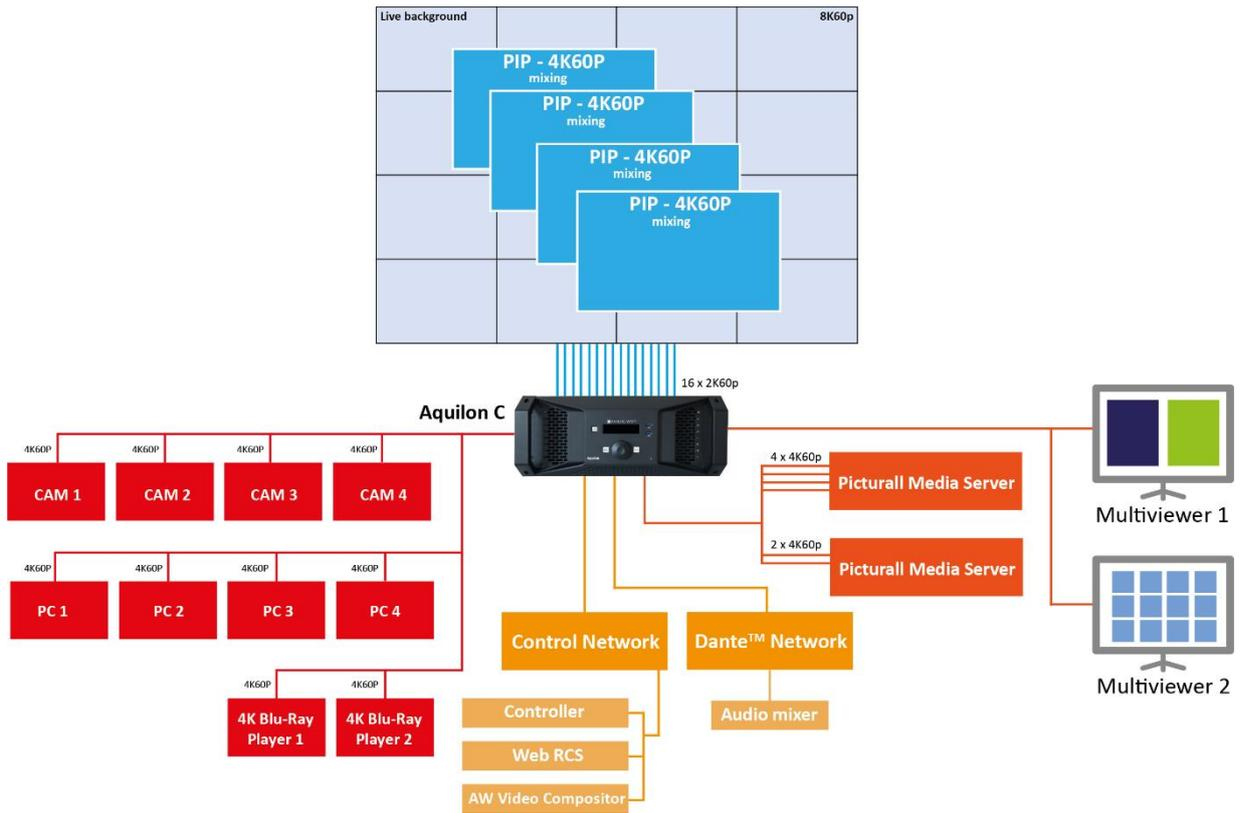
A single fully loaded Aquilon C can drive 2x 8K60p LED walls and 8x 4K60p AUX outputs
