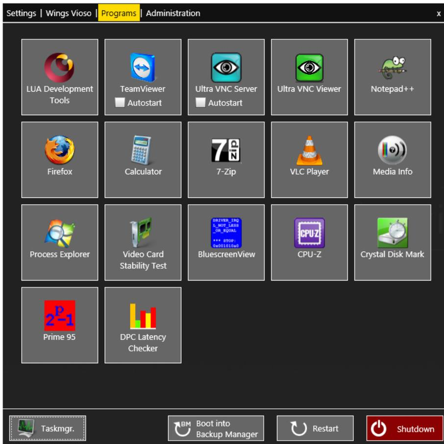
*Ultra VNC Server*: starts the Ultra VNC Server to allow remote support on the local network. You can activate the *Autostart* checkbox to offer this remote support functionality on system startup.
