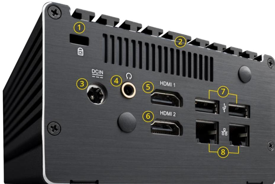
Details to ②: The cooling fins act as passive cooling for the dustproof case.
