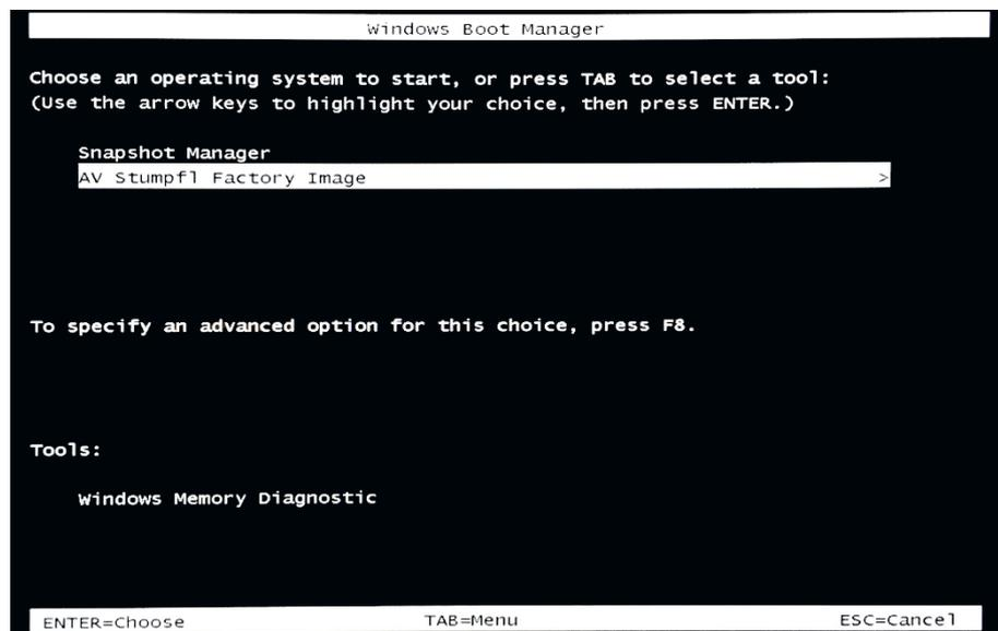
Select the entry *Snapshot Manager* and press the *Return* key which then lets the system boot into the Backup Manager.
