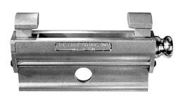
The Mega-Beam Clamp is a low profile sliding jaw design that allows you to secure your load as close to the I-Beam as possible. The 8" model has a 3 ton rating. The two aircraft aluminum jaws are adjusted on the 3/4"-6 tpi Acme threaded shaft. The spring loaded handle locks after adjustment. Aluminum construction is half the weight of steel units and has a wider gripping range.
