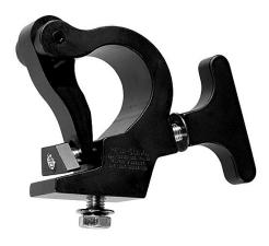
The new standard truss clamp for hanging intelligent lighting fixtures. Allows one man to hang intelligent fixtures. Simply flip the link up, place clamp over the pipe and the Mega-Claw holds the weight of the fixture for you while you secure it with the solid 3/4" thick handle. The Mega-Claw will fit onto (I- I/2" Pipe) 1.9" OD to 2" OD.
