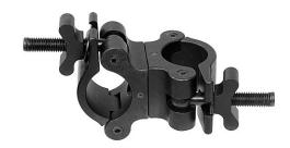
The Mega-Coupler will fasten from I-I/4" pipe (I.660" OD) to 2.050" OD truss tube. The Mega-Coupler has the wide wing nuts for fastening the clamp to the pipe or tube. Safe Vertical Working Load 1100 Pounds, (500 KG).
