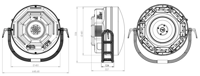
Dimensions of the circular housing: 481 x 481 x 327 mm<sup>3</sup>
